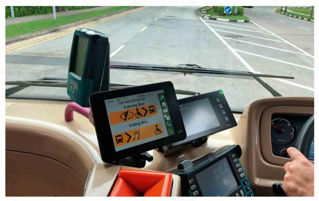
Unique to the init solution: drivers are notified when passengers with special needs wish to get on or off.
